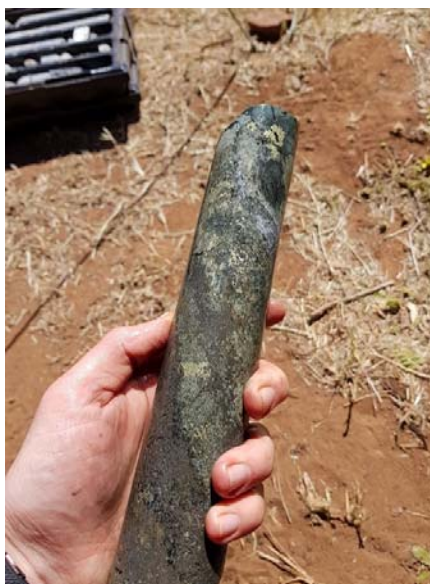
Drill core is from KPDD002 from 230.5m, showing pyrrhotite & chalcopyrite mineralisation within calcisilicate alteration
